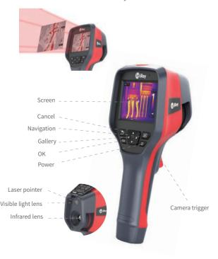
Manual focusing provides clear images of targets from far to near. Especially for observing tiny near targets. The lens equiped on M300 is close to the quasi macro level, so tiny targets at the size of 1mm (at the distance of 0.1m) can be distinguished.
