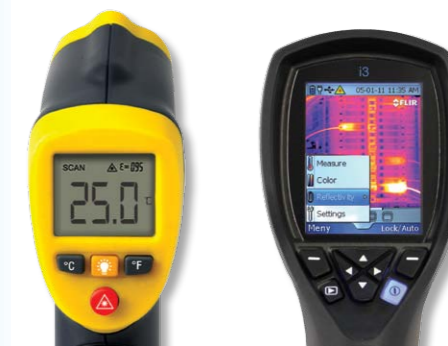
Spot pyrometer, temperature measurement in one spot.
